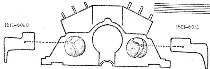
The above illustration shows the installed position of the baffles. The baffles should be pre-formed (bent) to the approximate contour they will have after installation. In order to achieve this with a minimum of exasperation, make yourself a pair of dummy cardboard baffles & use these to familiarize yourself with the installed position.
