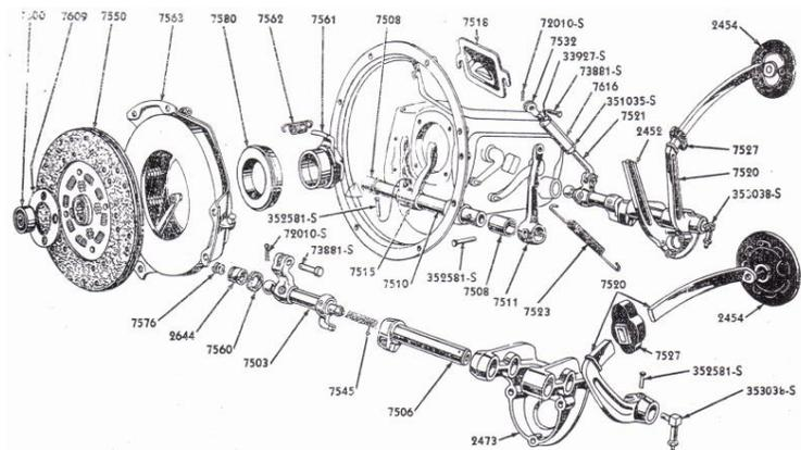
CLUTCH AND CLUTCH PEDAL (1940)
