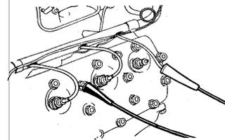
TESTING COIL OUTPUT, OPR. 12024-A
